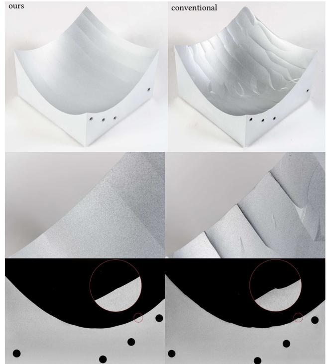
Fig. 14. Comparison of our curvature adaptive milling results (left column) with a conventional method (right column, cf. also Sec. 3.2.1). Our method (see Sec. 3.2.2) results in a much smoother surface as confirmed by the zooming (second row) and the planar section transversally to the tool path motion (third row). Aside: Visualization of our computed tool paths.
