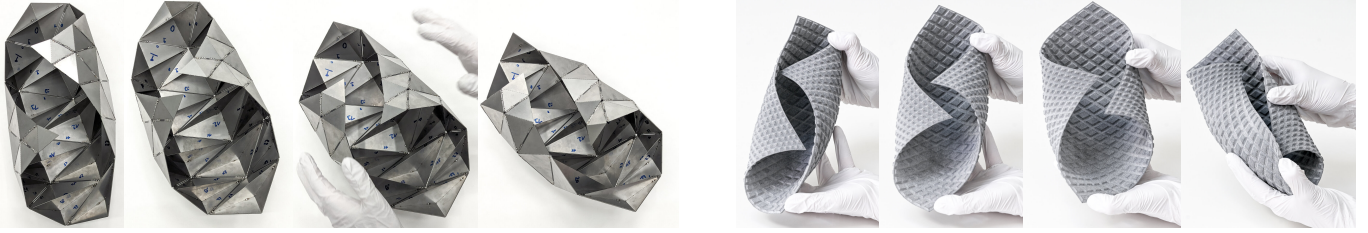
Fig. 23. Two flexing meshes (nonplanar quad case) approximating the same bending surface. Optimization here was based on the method of § 4.3.3. On the left we show the flexion of a 5 \times 5 precision model fabricated from faces with hinges in the way described by Fig. 22. The model with 20 \times 20 faces on the right has been 3D printed on a HP Multi Jet Fusion 3D Printing system using thermoplastic polyurethane. The material is flexible (Shore A hardness 88) but harder than the rubber of a typical automobile tire (Shore A hardness 70). The model has a thickness of 4 mm that is reduced to 0.6 mm at the joints. The resulting local reduction in stiffness creates a well-defined flexure bearing. Note that the 3D printed version still exhibits only the flexibility that was computed on the basis of rigid faces and hinges in the edges. This is shown by our actuating the model on the right hand side only and observing that the left hand side automatically moves as computed.
