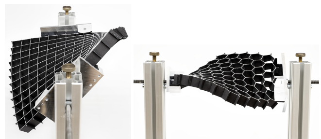
Fig. 22. Verification of the C-mesh property by means of scanning physical models. Edge lengths are 20 mm (quad case) resp. 14 mm (hex case).
