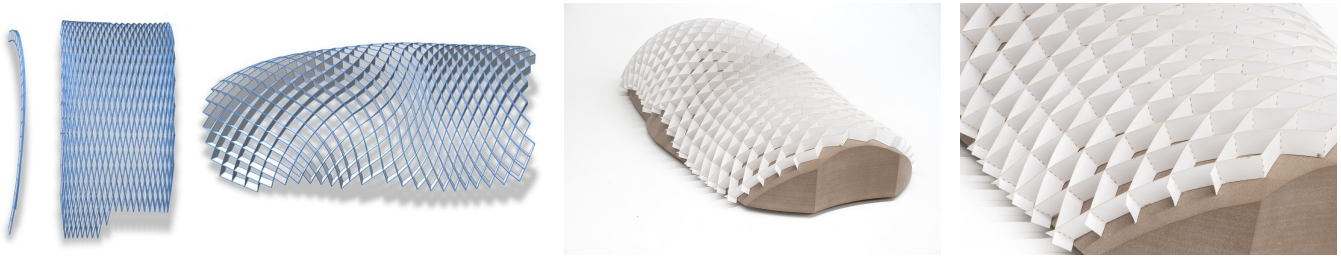
Fig. 20. Deployment of a quadrilateral C-mesh from a circular polyline, and an actual paper model of this mesh made from lasercut strips assembled manually. For an animation of the continuous deployment we refer to the accompanying video.
