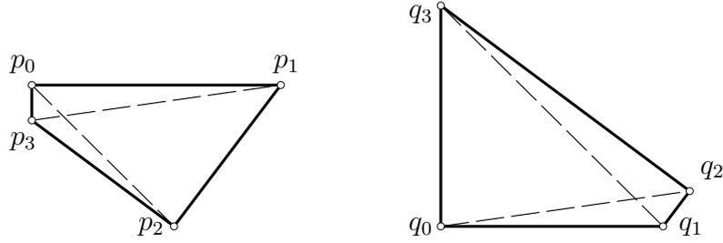
FIGURE 9. A pair of parallel quadrilaterals  $p_0, \dots, p_3$  and  $q_0, \dots, q_3$  has vanishing mixed area if and only if their non-corresponding diagonals are parallel:  $q_0q_2 \parallel q_1q_3$  and  $q_1q_3 \parallel q_0q_2$ .
