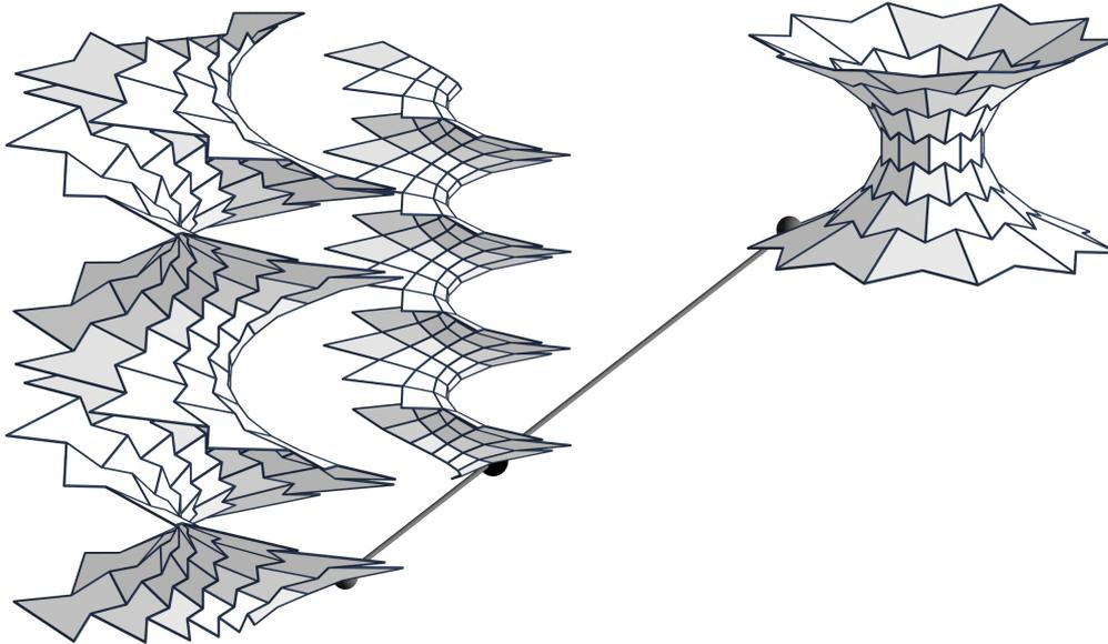
FIGURE 7. Linear combinations of parallel meshes, where one is a discrete catenoid and the second is a discrete helical surface are members of the corresponding associated family of minimal surfaces. Special combinations can lead to quad meshes. The case illustrated here is in fact a discrete helicoid, which means that it discretizes a surface generated by the helical motion of a straight line which orthogonally intersects the helical axis (see Example 4).
