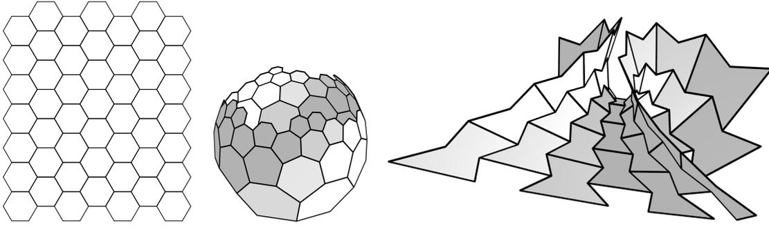
FIGURE 12. *Left:* Circular conformal mesh which discretizes  $z \mapsto z$ . *Center:* Discrete Gauss image, which is the stereographic projection of the circular conformal mesh. *Right:* Discrete minimal surface generated as the discrete Christoffel dual of the Gauss image. According to Example 1 the hexagonal mesh is a discrete Enneper's surface.
