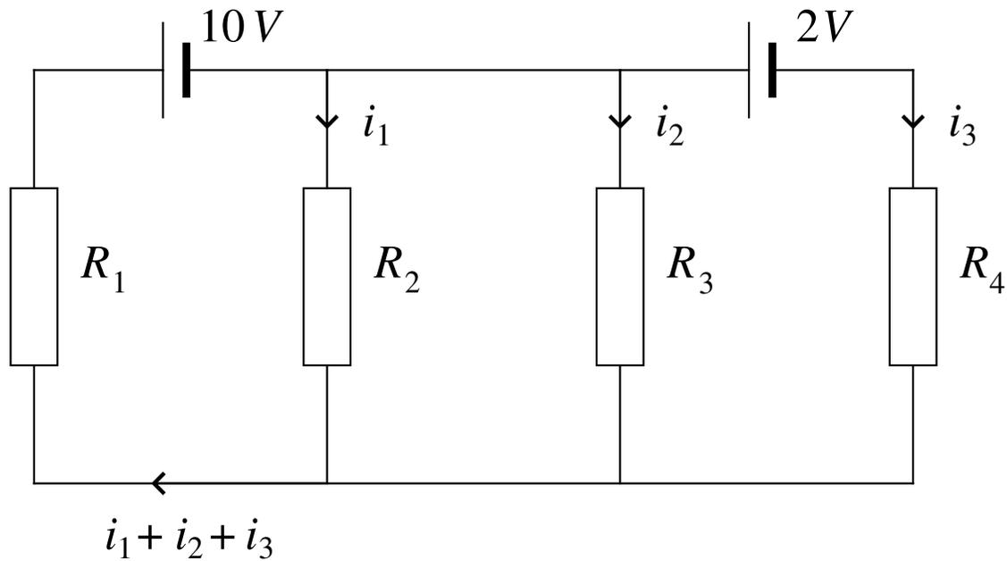
$$\begin{aligned} 5.5 i_1 + 1.5 i_2 + 1.5 i_3 &= 10, \\ -4 i_1 + 4 i_2 &= 0, \\ -4 i_2 + 3 i_3 &= 2. \end{aligned} \iff \begin{pmatrix} 5.5 & 1.5 & 1.5 \\ -4 & 4 & 0 \\ 0 & -4 & 3 \end{pmatrix} \cdot \begin{pmatrix} i_1 \\ i_2 \\ i_3 \end{pmatrix} = \begin{pmatrix} 10 \\ 0 \\ 2 \end{pmatrix}.$$
