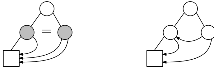
Fig. 2. (Left) The smallest relaxed binary tree that is not a compacted binary tree, as the two gray subtrees correspond to the same (classical) binary tree. (Right) A valid compacted binary tree of size 3 with the same spine.
